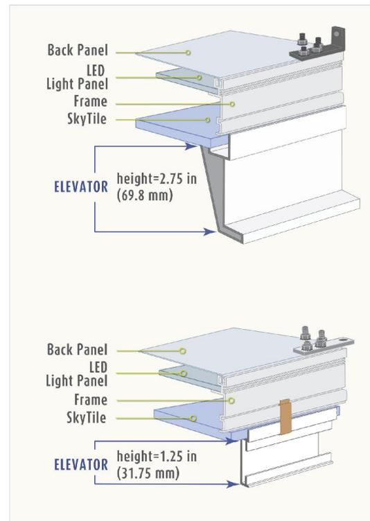
Standard Luminous SkyCeiling elevator
